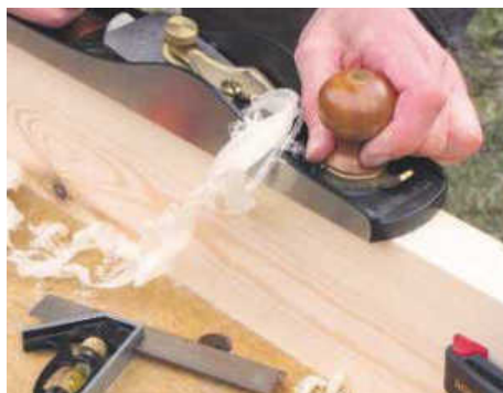
STEP 20. Cramp both shelves together and plane the sawn edges for accuracy. Sand faces and remove arrises
